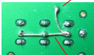
Center socket pins grounded together with part lead
