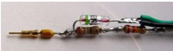
\*\* The ARRL probe uses a series .01 cap, 1n34a shunt diode and 4.7Meg scaling resistor. The handbook description also includes considerable rounding. The only change I made is the 4.1Meg scaling resistor.
