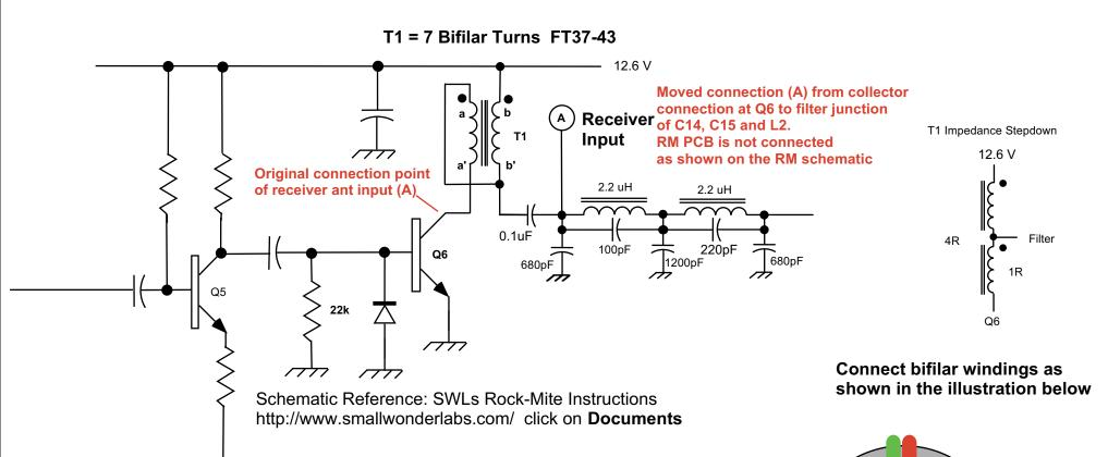
This bifilar transformer mod provides a better match to Q6 and the input of the filter. The results will be better efficiency with about 20% more output power. Because the efficiency is better, the PA will run cooler. A 30 sec keydown barely warms the Q6 heatsink
