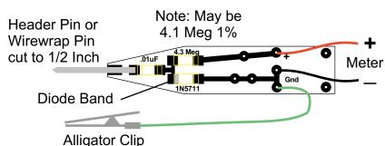
Tin pin and pads first and position at end of .01 cap and solder after the capacitor is in place.
