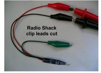
At QRP power levels, shielding is not a requirement. If holding the probe by the leads is not acceptable, a plastic tubing enclosure or clear shrink sleeving will do the job quite nicely.
