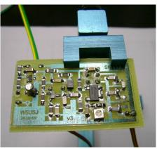
QRPkits.com supplies this really neat PCB holding vice. The board is positioned up about 5 in. and makes it easier to work on the assembly for positioning and soldering the parts. Doesn't help with shaky hands and keeping the parts lined up nicely. The clamp screws are on the bottom to keep them out of the way.
