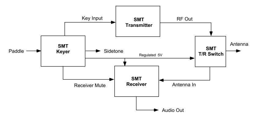
Note: 5V SMT regulators can be left off individual SMT Receiver and T/R switch assemblies and supplied as shown
