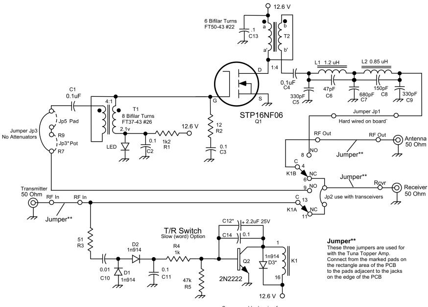
See assembly drawing for use of Jp4 for fast/slow T/R switch
