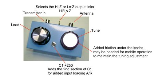
Tuning with the Z-Match is an iterative process.
